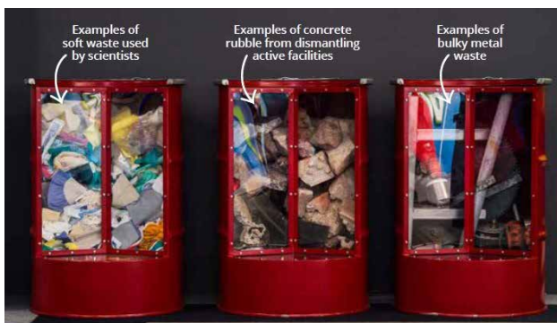
Example LLW drums, showing the types of waste that may be contained inside.
