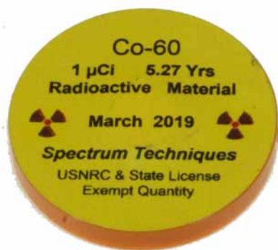
Cobalt-60 disc source, original activity of 1 µCi (37000 Bq), half-life of 5.27 years. Image courtesy of Industrial Equipment and Control Pty Ltd
