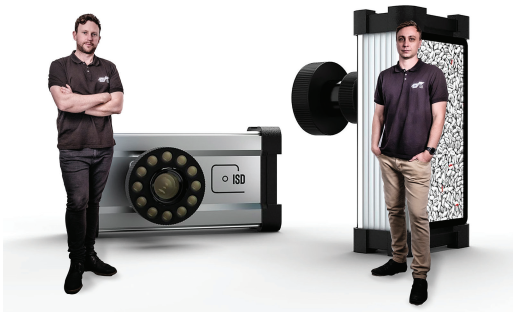
Co-founders Julian and Jason pictured with the Handheld Device developed by ISD, which utilises multiple sensors including hyper-spectral and RGB cameras. The onboard AI is capable of detecting pests in real time alerting operations and biosecurity staff. Image credit: ISD
