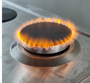
A sample cooktop burner running on 100% hydrogen.
