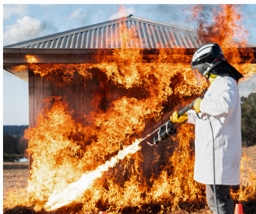
FIRECOAT external paint developed for extreme fire protection (left), FIRECOAT fire suppression and protection paint test (right)
