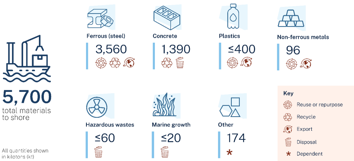
Figure 8: Materials predicted to be returned to shore for reuse, recycling, or disposal in Australia across a projected time frame of 2023–2060 and indicative material management pathways (CODA 2022b; CSIRO 2024a).
