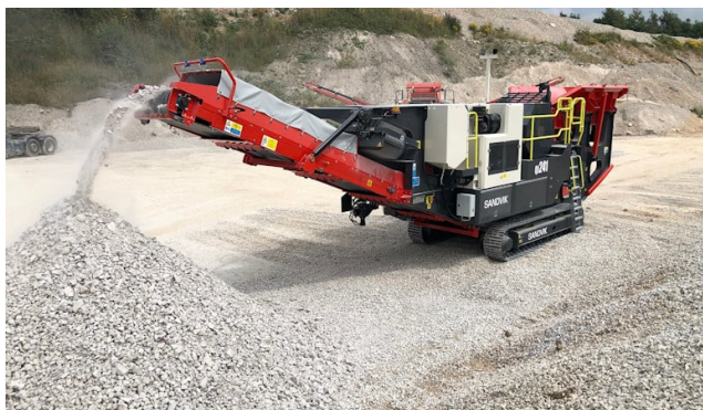
Figure 31: Mobile Crusher used for Creating Recycled Aggregate Products - Rock Processing Solutions
