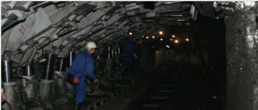
Figure 4.15 - Longwall face supported by mechanized shields, extracted by the shearer applied at Vangdanh coal mines in 2007
