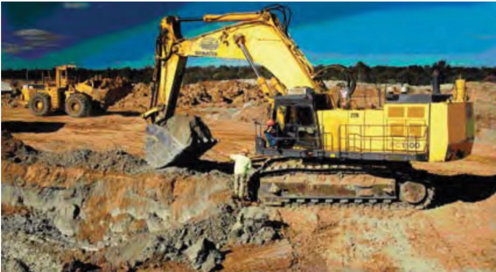
Figure 4.9 - Geological control to separate acid generating material
