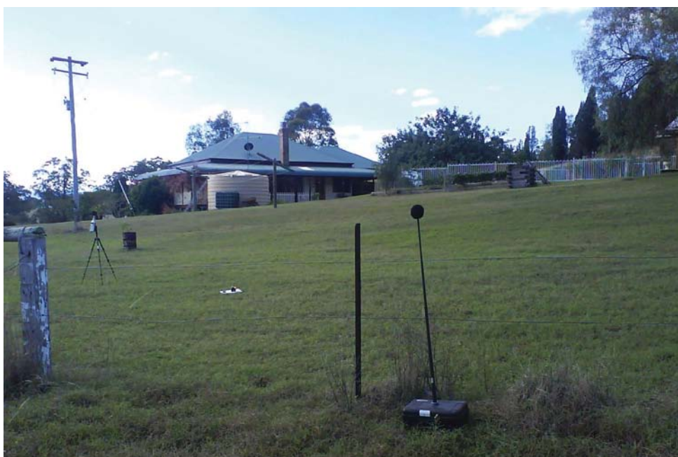
Figure 2.2 - Example of environmental noise logger in operation.
