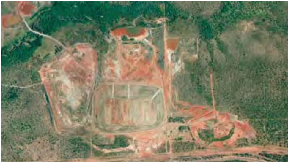
Figure 5.19 - Rehabilitated mine site in 2005, following construction of cover over the waste rock pile.
