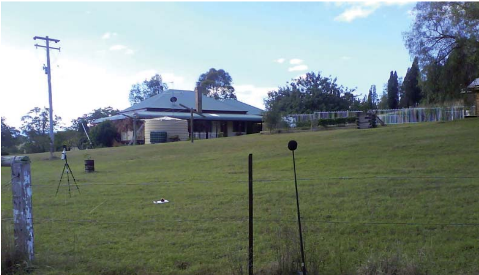
Example of environmental noise logger in operation. Source: Wilkinson Murray.
