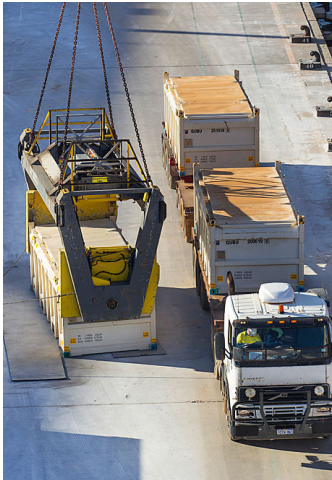
Bulk transport of metal concentrates using sealed containers and rotating spreaders.
