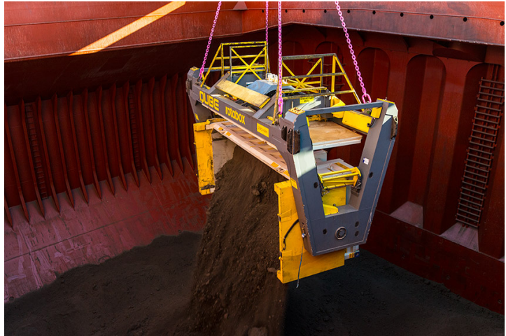
Bulk transport of metal concentrates using sealed containers and rotating spreaders.
