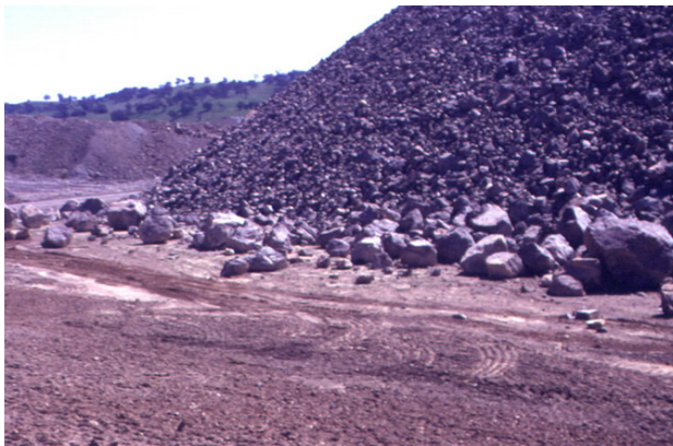
Figure 20: Base rubble zone (top); angle of repose and trafficked layers (bottom)
