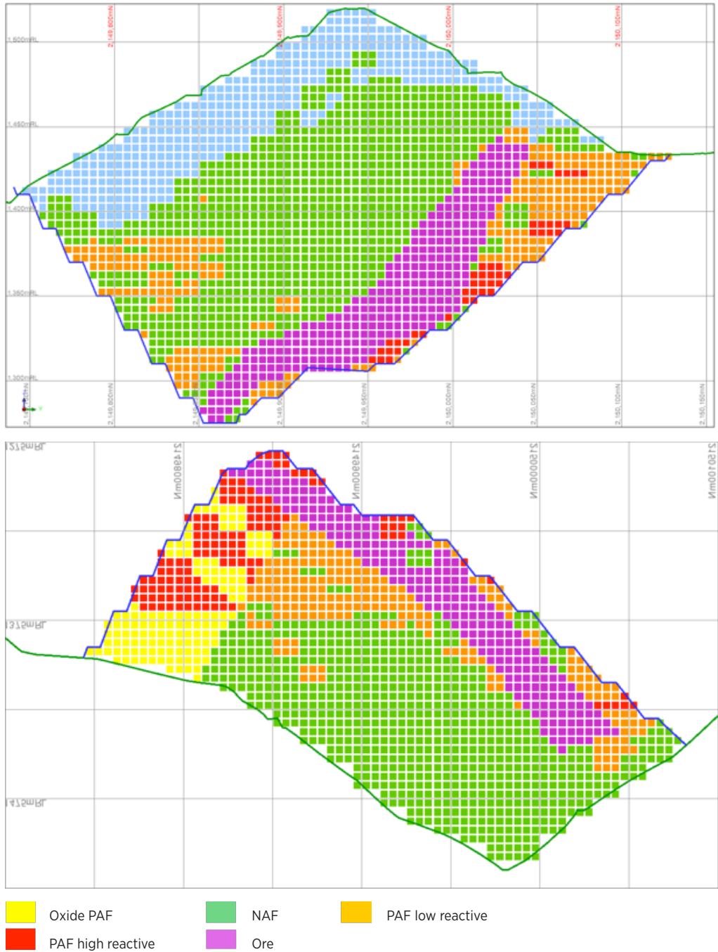
Figure 10: Visual representation of an AMD block model—two slice cross-sections showing relationship of waste types to proposed open-pit shell (ore body shown in purple)
