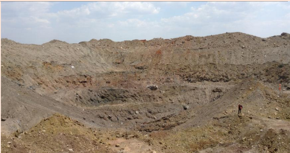
Figure 2: Excavated sampling pit (15 m bench level) in the Main WRD. Scale is provided by a 2 m person standing on the right-hand side
