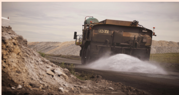
Water being sprayed on a mine haul road to reduce dust at a Hunter Valley mine.
