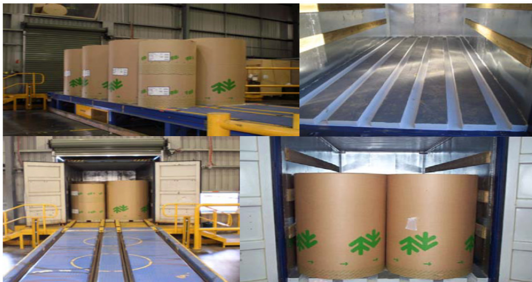
Figure 1: Skate loading systems at the Boyer Mill
