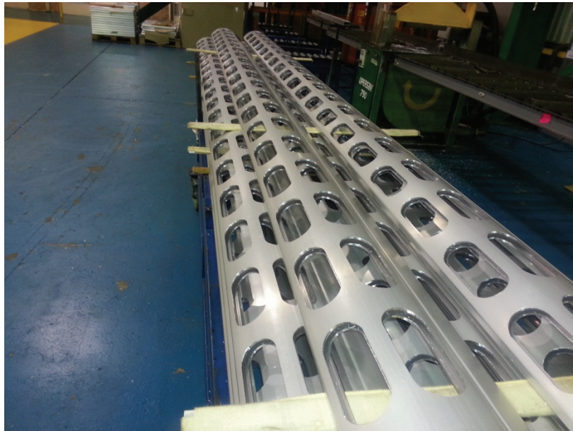
Application: Transport – Air-conditioning duct
