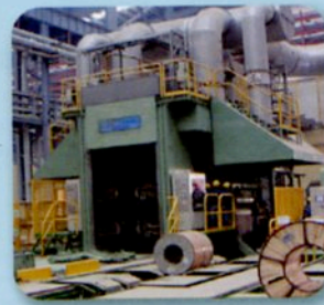
冷軋機 (CRM) 6-Hi, Reversing Cold Rolling Mill
