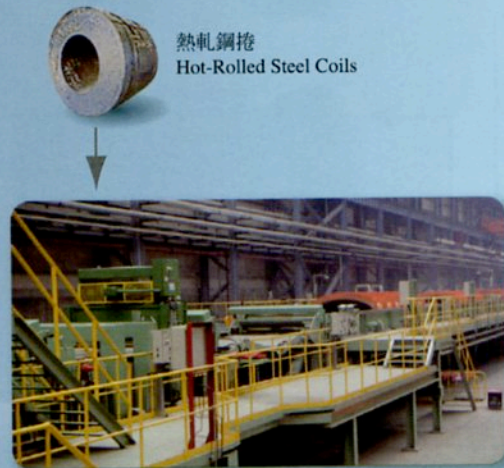
酸洗線 Push-pull Pickling Line
