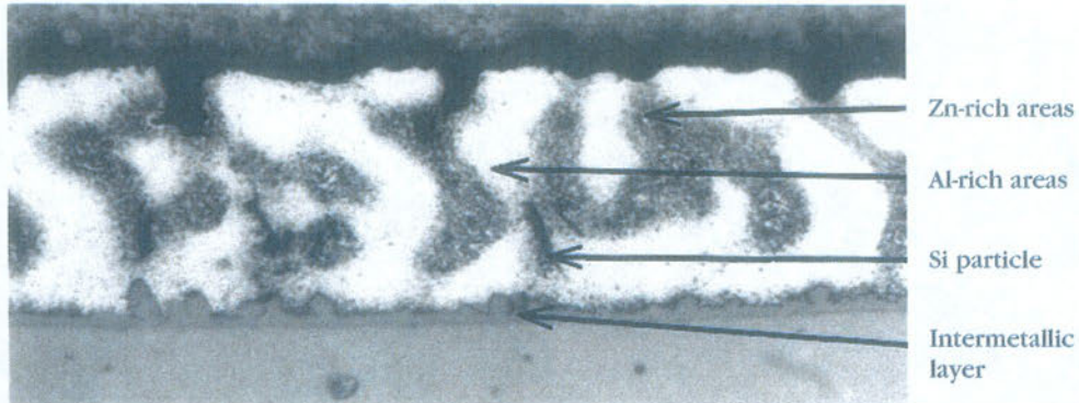
Figure 1: ZINCALUME® Steel Microstructure
