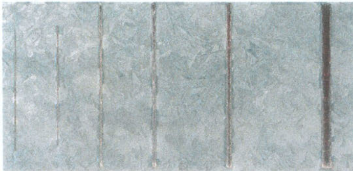
Figure 4: Zinc-coated sample, Z275.
