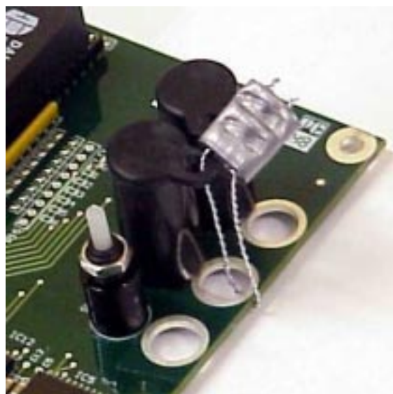
Sealing of Meter Calibration (K-factor) Switch
