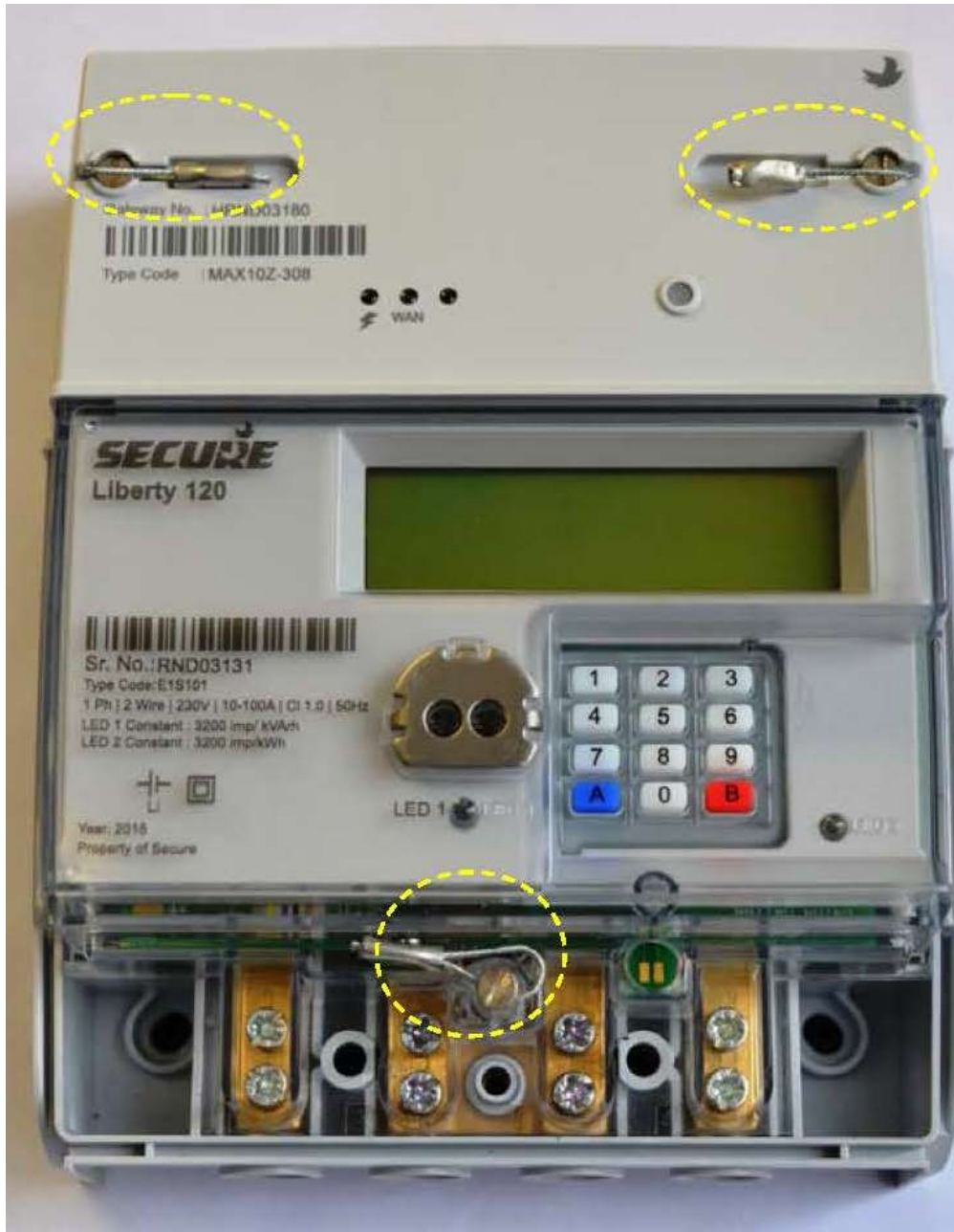
Model Liberty 120 Showing Typical Mechanical Sealing
