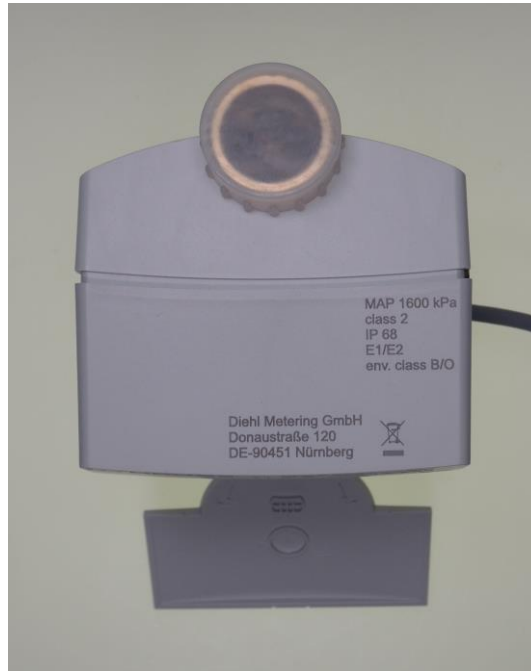
Example of required markings (continued) on side of case
