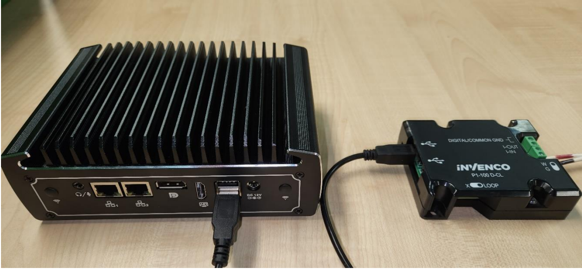
Invenco Model C1-100 Controller operating on an Industrial PC with separate Pump Interface board (Variant 1)
