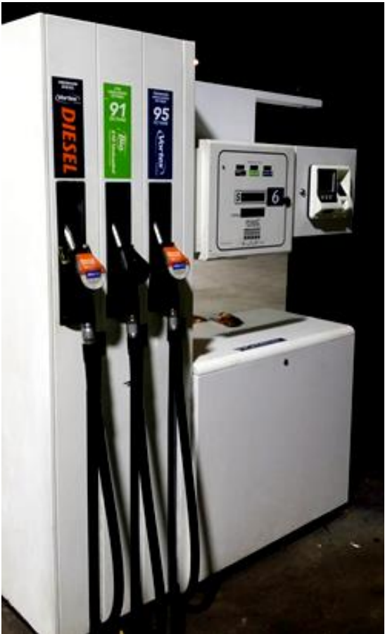
Typical Invenco Model G6 6525X Terminal Installations in Various Fuel Dispensers
