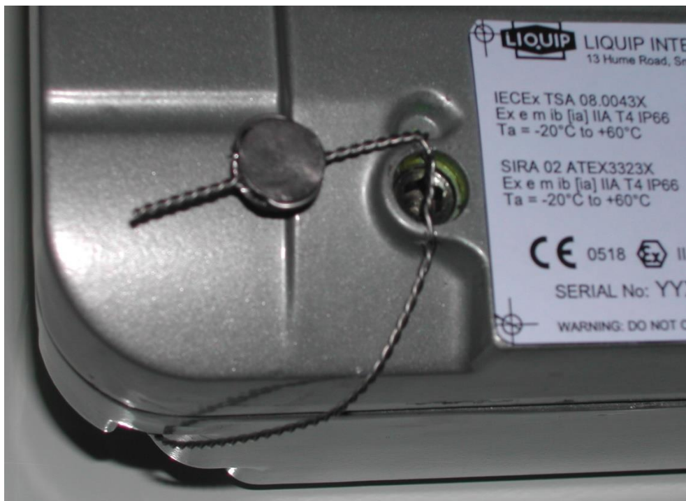
Typical Sealing of the DFV1** Cal Button to a Cover-mounting Screw (not shown)
