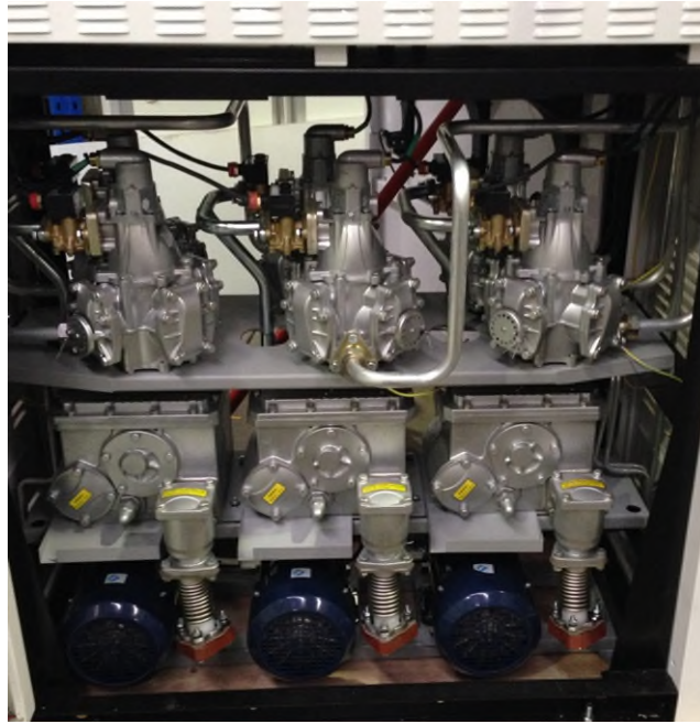
Typical Version 56 Dispenser Hydraulics (Variant 1)
