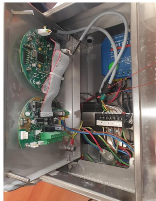
Placement of ferrite clamps – Variant 7
