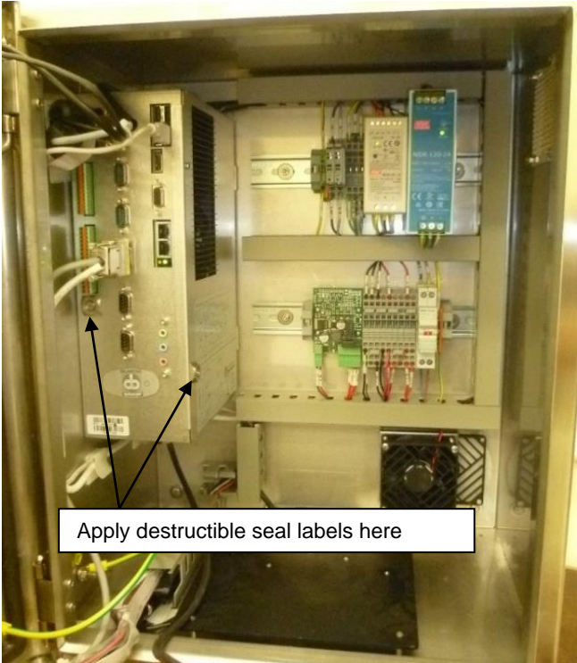
(a) Typical Hardware Seal of DD2060 Indicator
