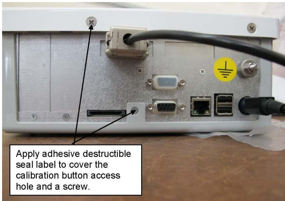
Typical Hardware Sealing of Models DD1010H & DD1010 (Variants 3 & 5)
