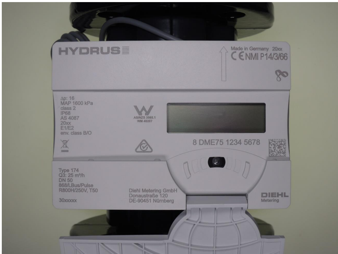
Example of indicating device and required markings
