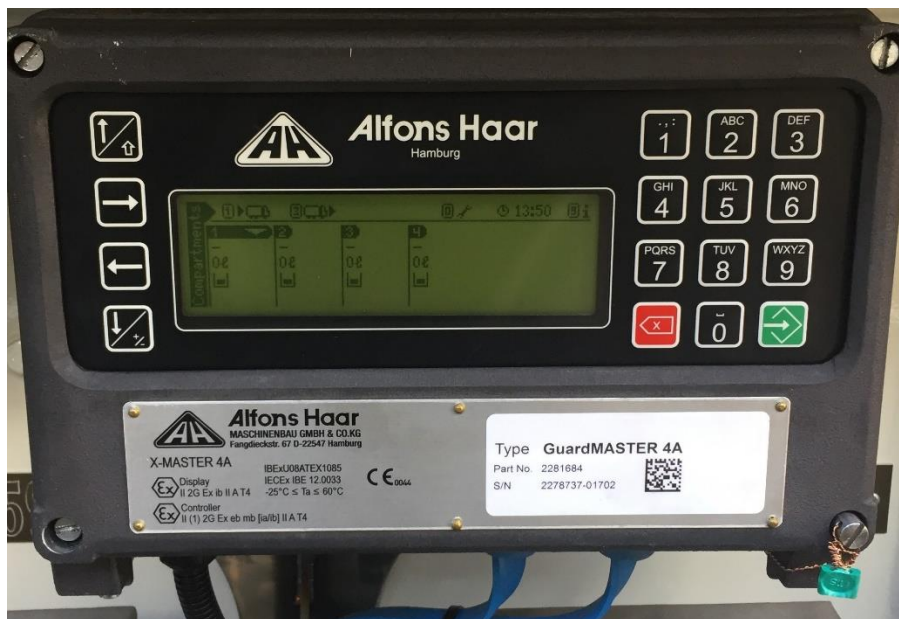
An Alfons Haar Model CountMASTER 4A Calculator/Indicator Unit (also known as GuardMASTER, ARUMASTER)
