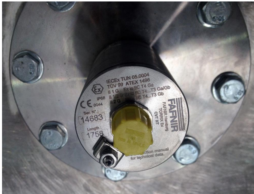
A FAFNIR Model 908734-XXX Series Electronic Dipstick
