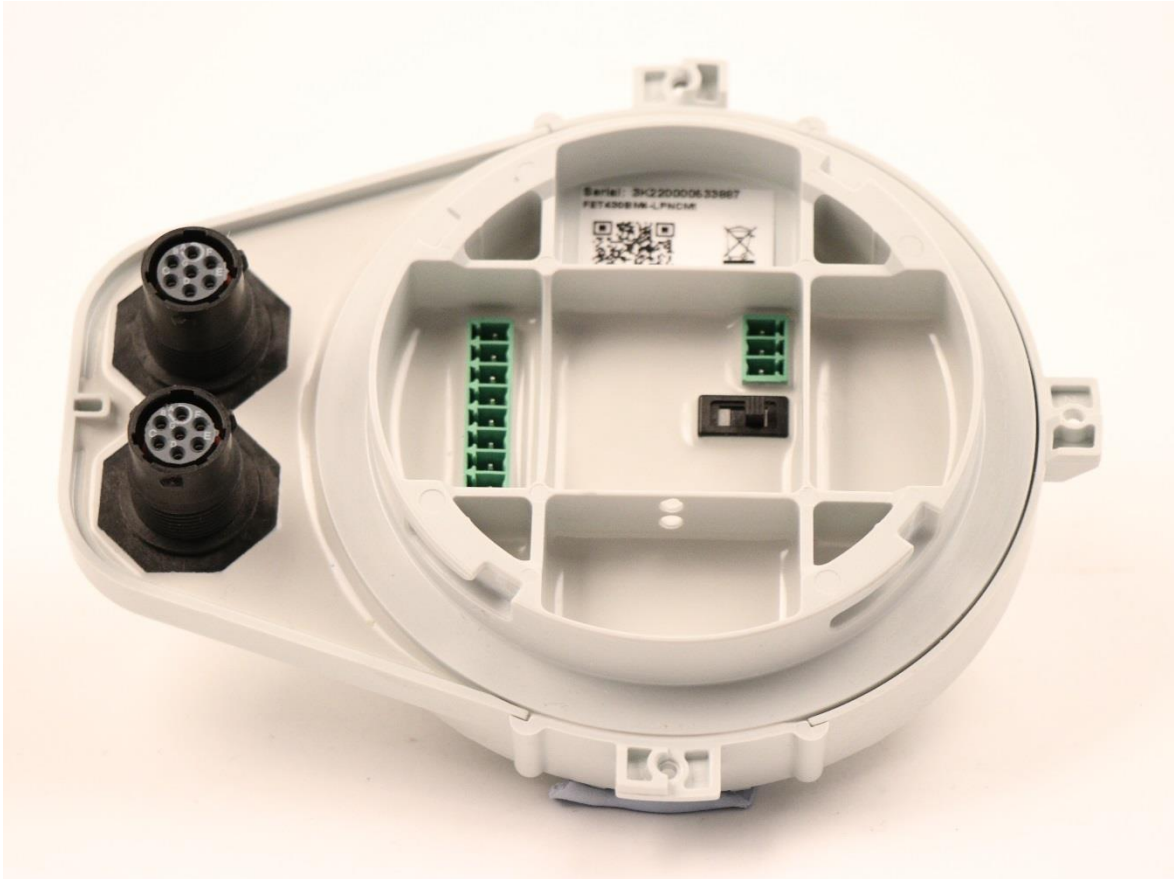
AquaMaster4 – Sealing Device: read-only switch
