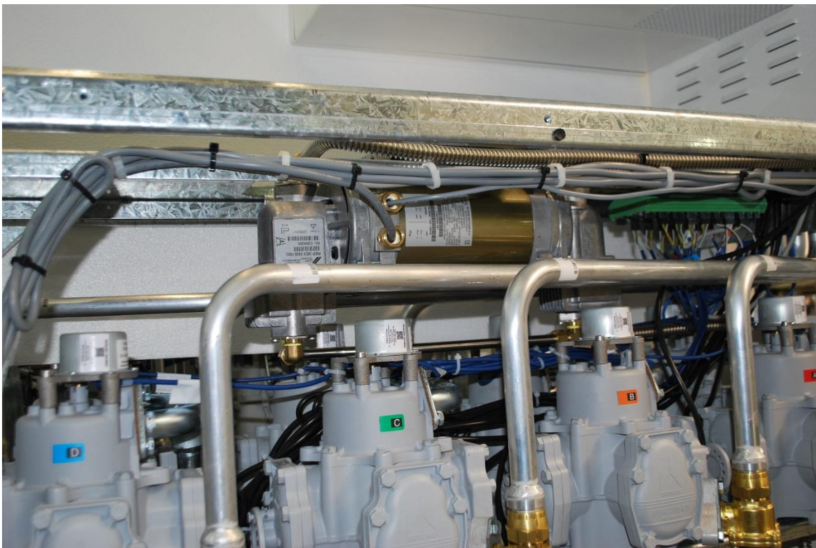
Tatsuno Model MP-02515 Meters With Pulse Generators – The Pattern (Also Shows a Vacuum Pump – Variant 4)
