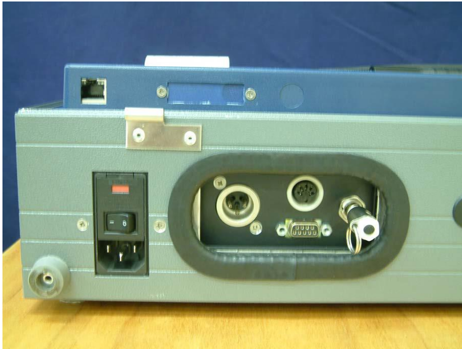
Showing a Typical Ethernet Port (Variant 1)
