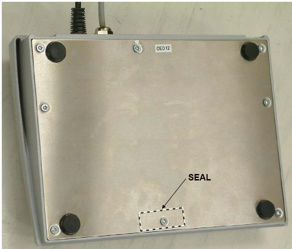
(b) Sealing of IND 439 Control/Indication Unit
