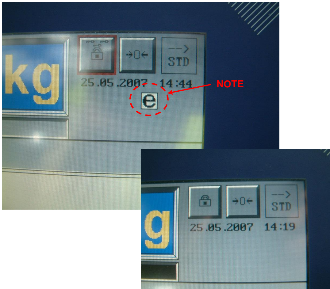
(b) Protection of Metrological Parameters
