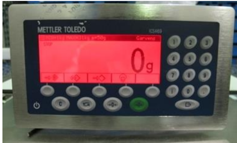
Alternative Garvens (or Mettler Toledo) 'ICS 4x9d' or ICS 6x9d' Series Control/Indication Unit
