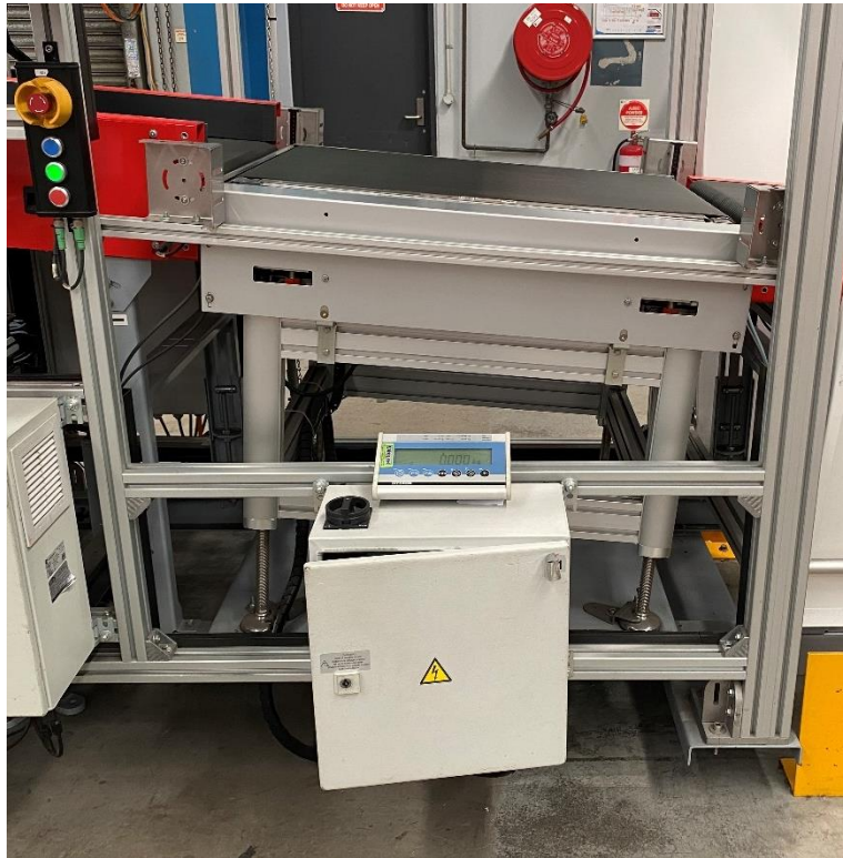
Bizerba Model CWL-I Automatic Catchweighing Instrument Load Receptor in Tilted Position (Variant 9)
