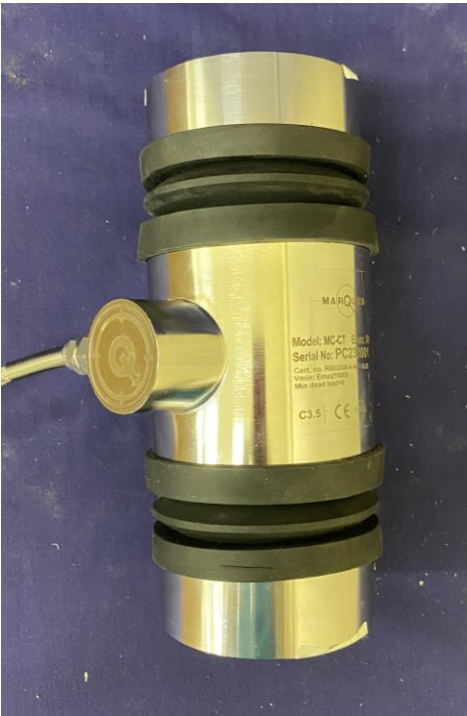
Marques Electronic Technology Model MC-CT Load Cell With Rubber Bellows Fitted
