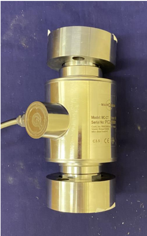
Marques Electronic Technology Model MC-CT Load Cell (Note: Use without the rubber bellows is acceptable)
