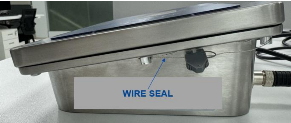
Mettler Toledo Model IND360 Harsh Version 'Lead & Wire' Type Sealing Method (Variant 2)
