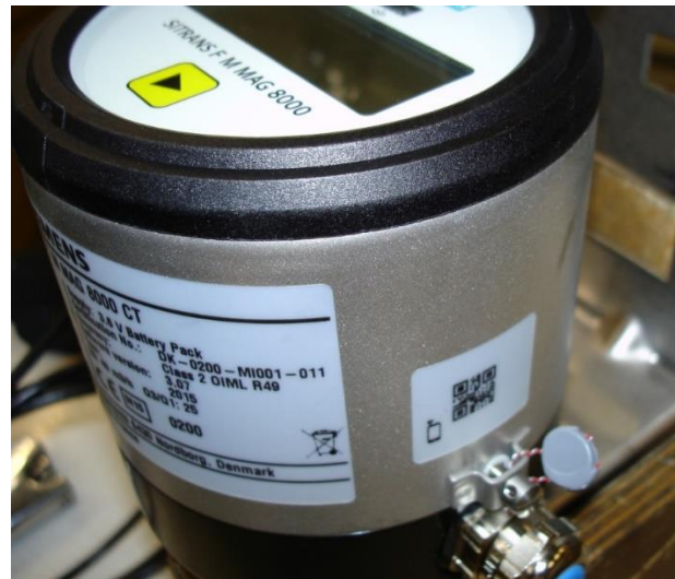
Typical Mechanical Sealing of MAG8000
