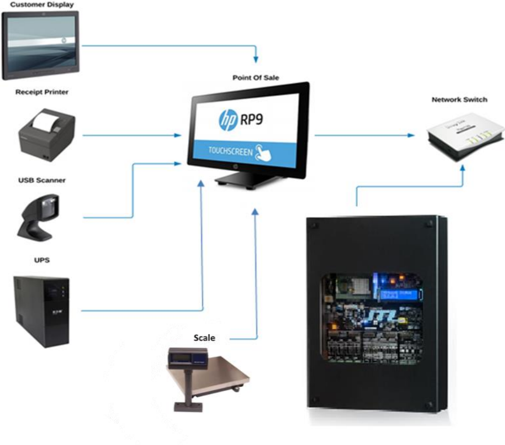
Point of Sale (POS) System configured for Self Service Fuel and Point of Sale weighed items (Variant 4)
