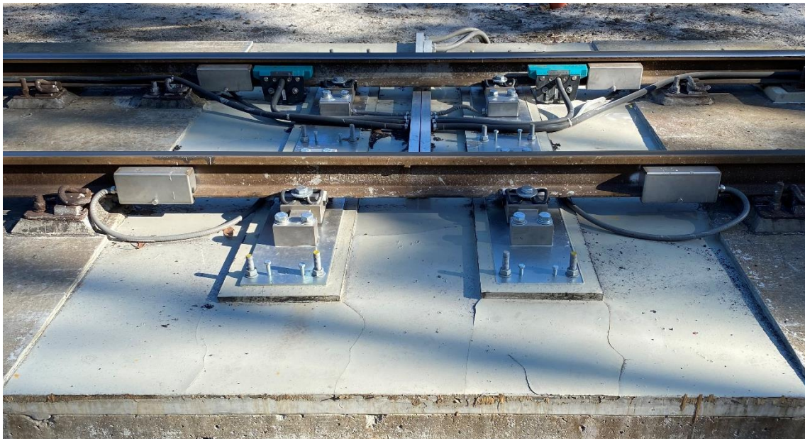
Infinity LS System Load Receptor Incorporating Steel Sleepers and Lateral Force Sensors
