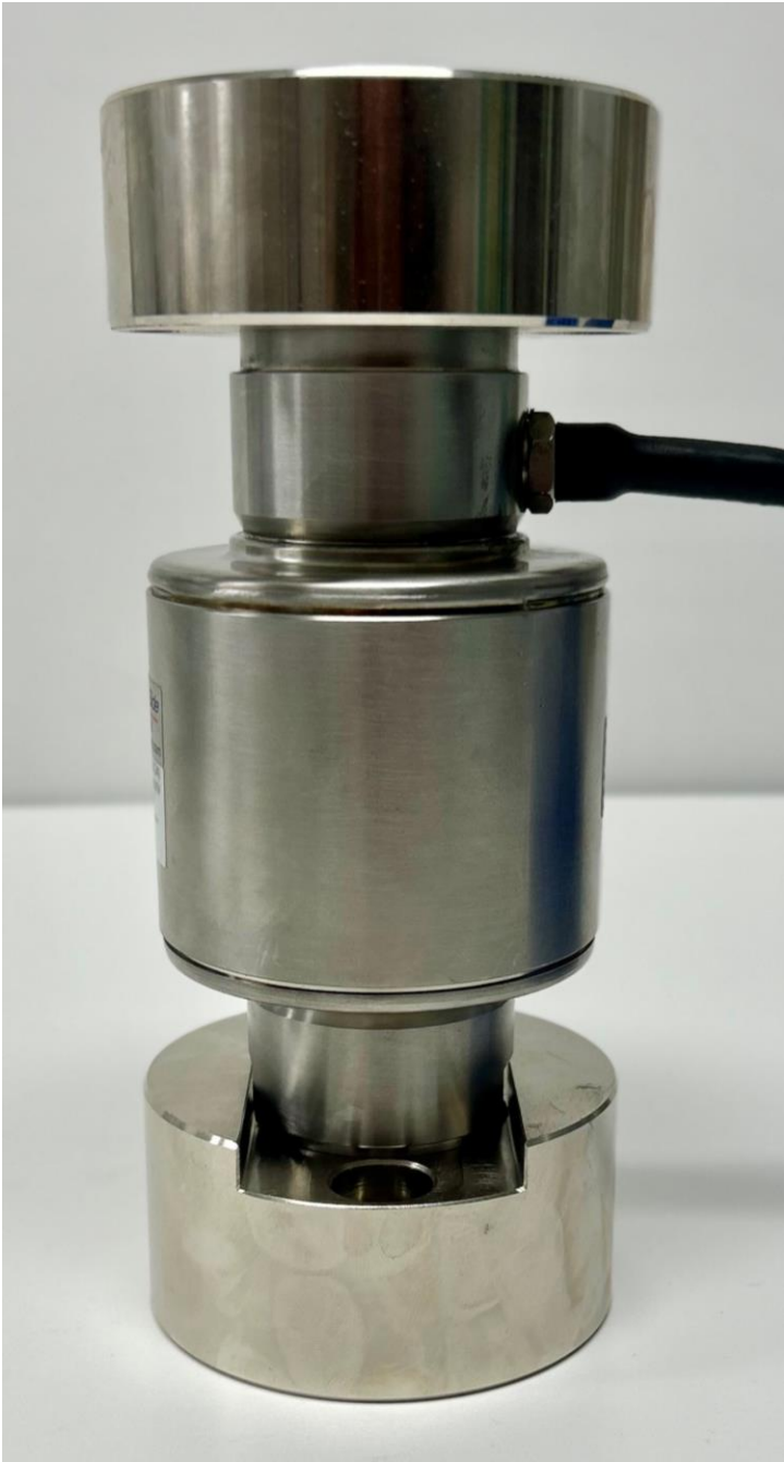
Typical Mounting Arrangement for T34X Load Cell
