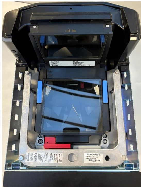
(b) Datalogic Model Magellan 9554 Weighing Instrument With Load Receptor Plate Removed (Variant 2)
