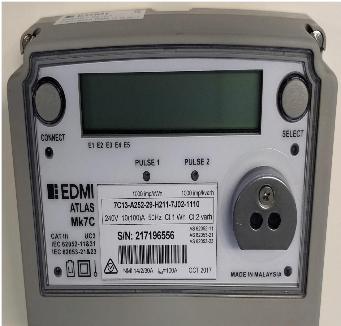
Variant 2 of EDM I model Mk7C Class 1 Electricity Meters showing the manufacturing code '7C13'
