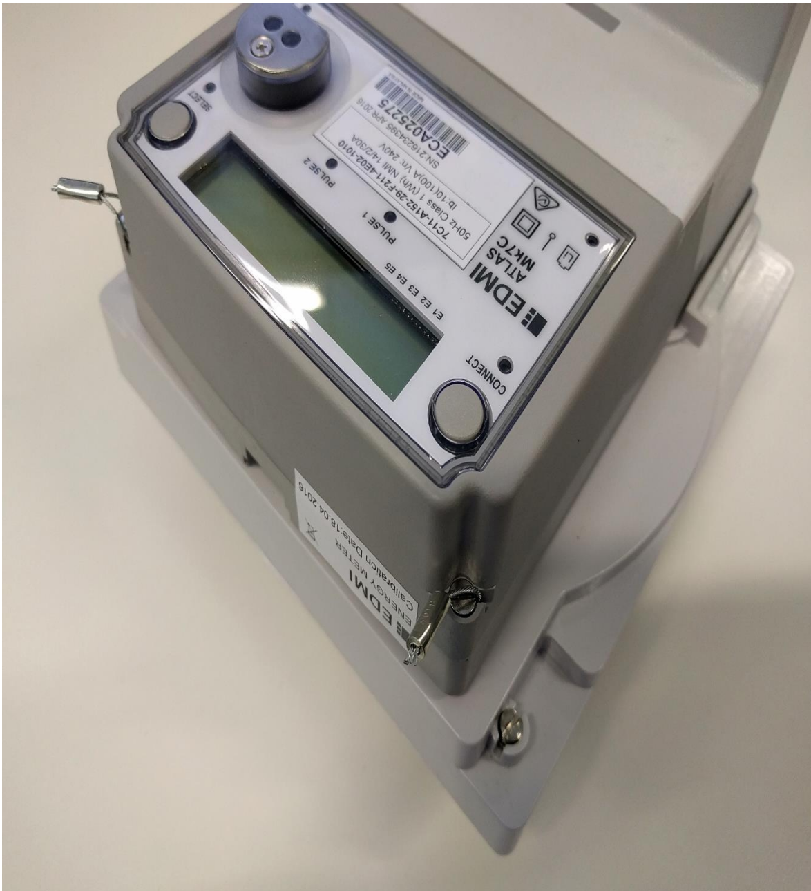
Variant 3 of EDM I model Mk7C Class 1 Electricity Meters with the plug-in base adaptor
