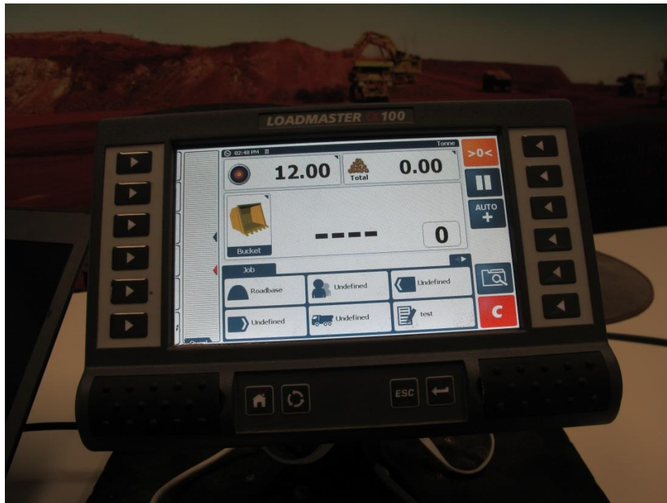
Loadmaster ISOCAN Control and Display Unit (Pattern)
