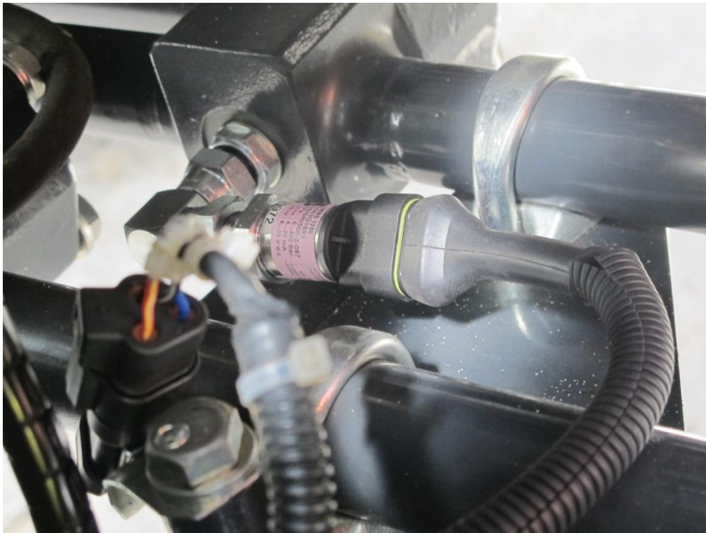
Typical RDS Pressure Sensor Installation
