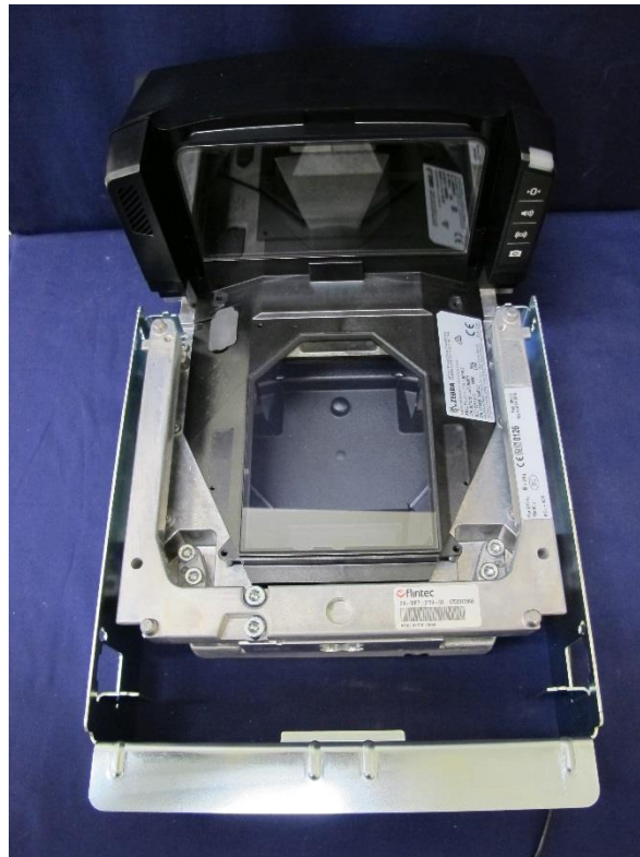
(b) Zebra Technologies Models MP70X1 & MP70X2 Series With Load Receptor Plate Removed (Pattern)
