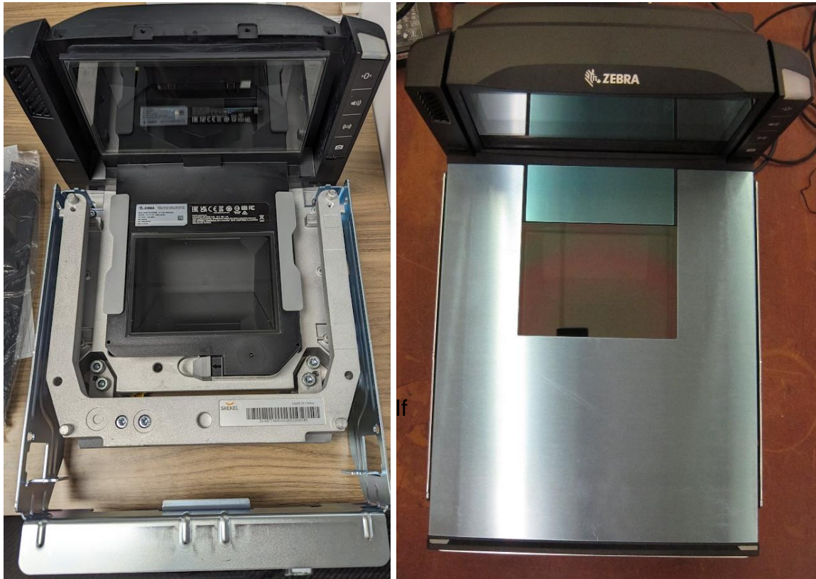
Zebra Technologies Models MP72X1 & MP72X2 Series Weighing Instruments With Load Receptor Plate Removed (Variants 8 & 9)
