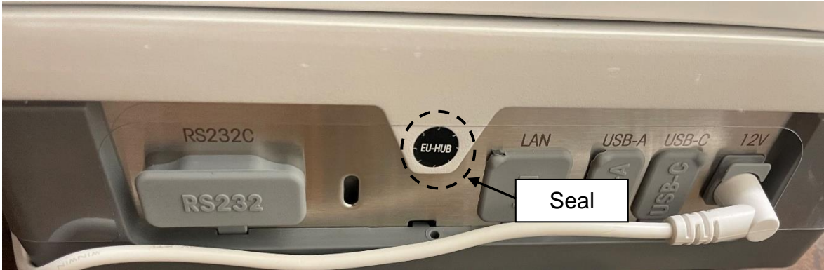
(a) Sealing Arrangement Using Destructible Adhesive Label
