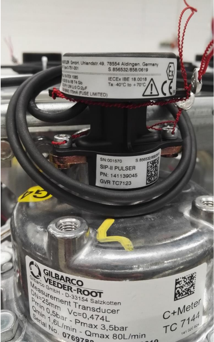
Gilbarco Model SIP-II Pulse Generator (incl. typical sealing method) – Variant 1
