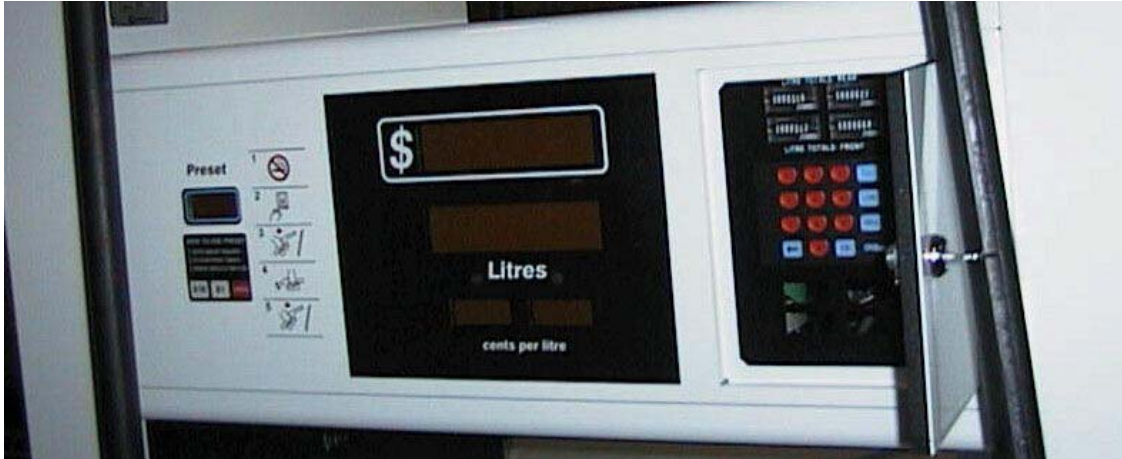
Gilbarco Model Epsilon Indicator/Calculator Module in 'Narrow Frame, Lane Orientation' Dispenser
