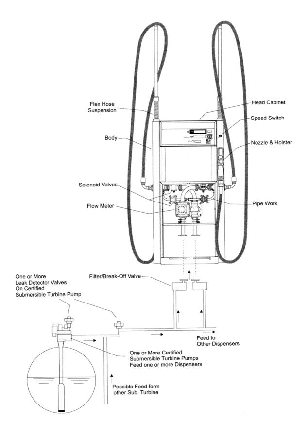
Typical Submersible Turbine Pump System
