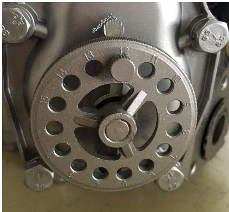
(b) Typical Sealing of Flowmeter
