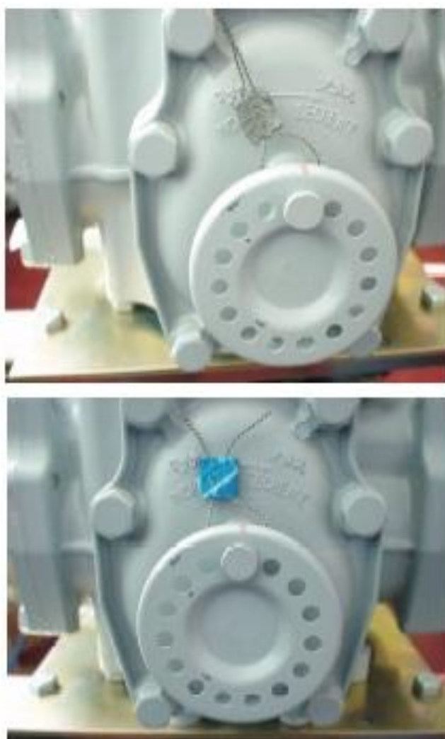
Typical Sealing Methods – Tatsuno Non-LPG Meter – The Pattern
