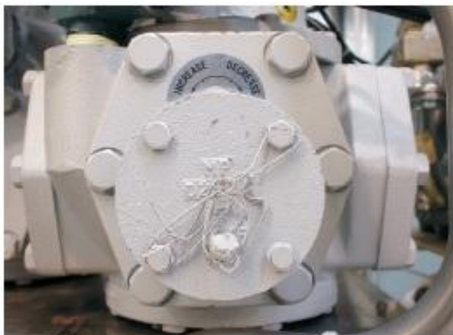
Typical Sealing Method – Tatsuno LPG Meter – The Pattern
