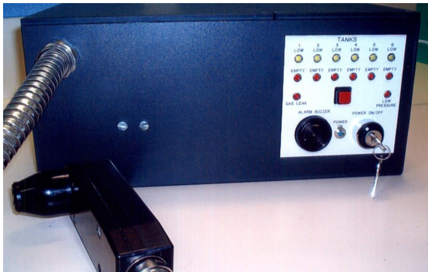
(b) Control box front view with status LEDs
