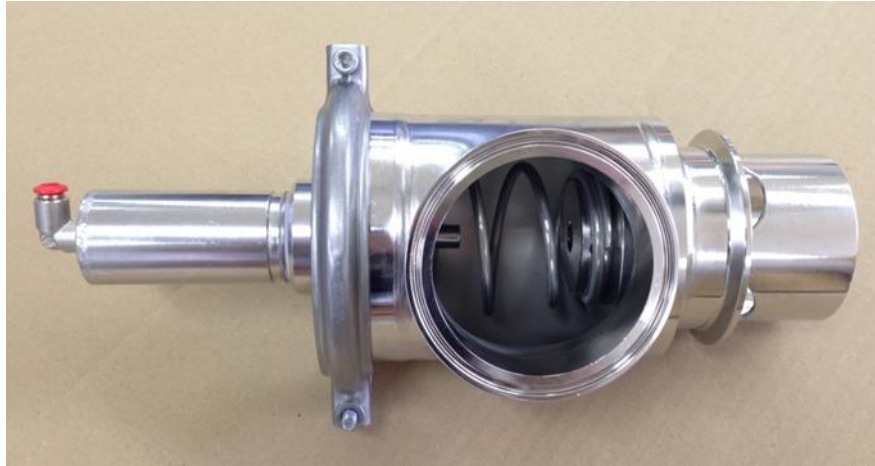
b) Poul Tarp Model 018302641001 Air-Operated Non-Return Valve
