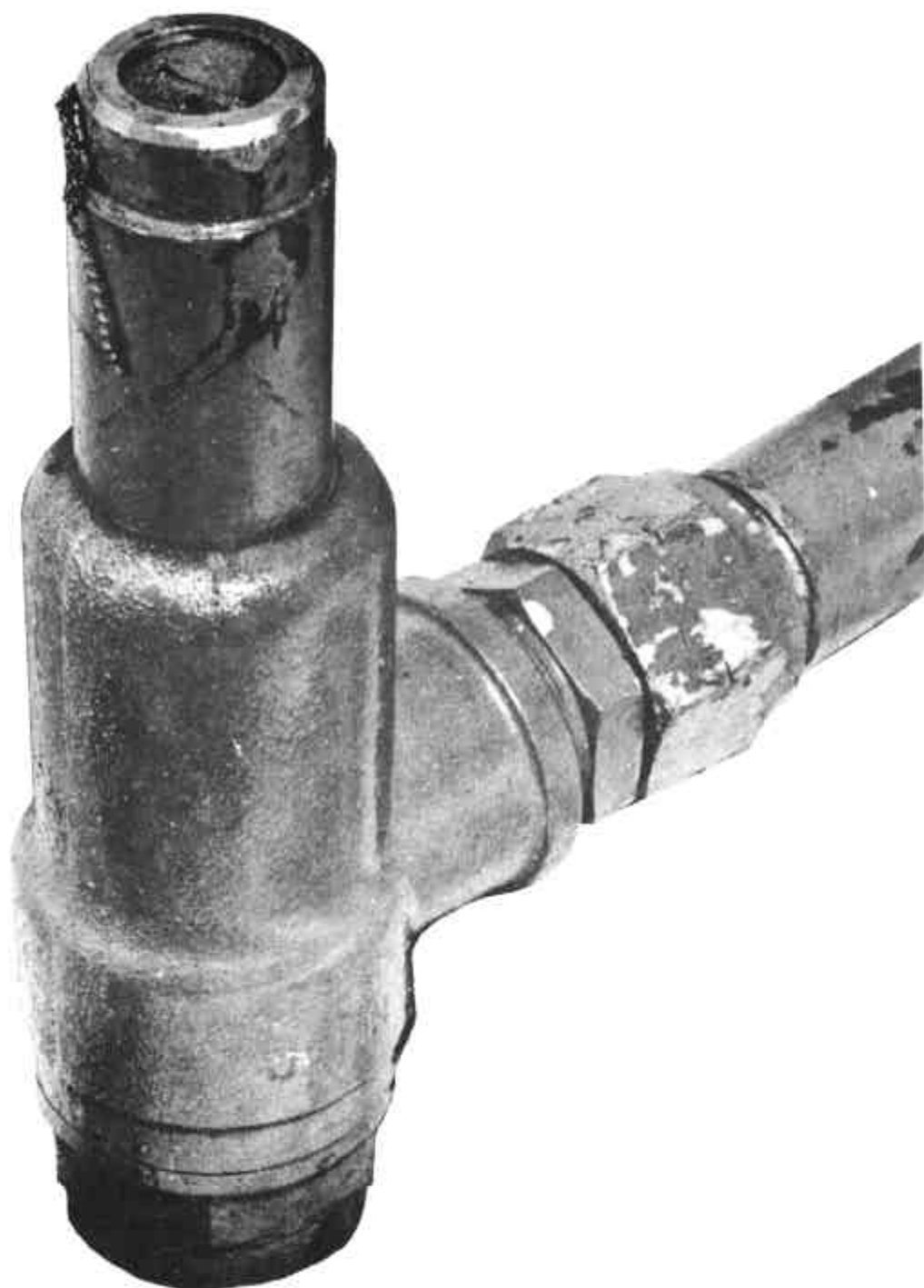
Pump By-pass Valve
