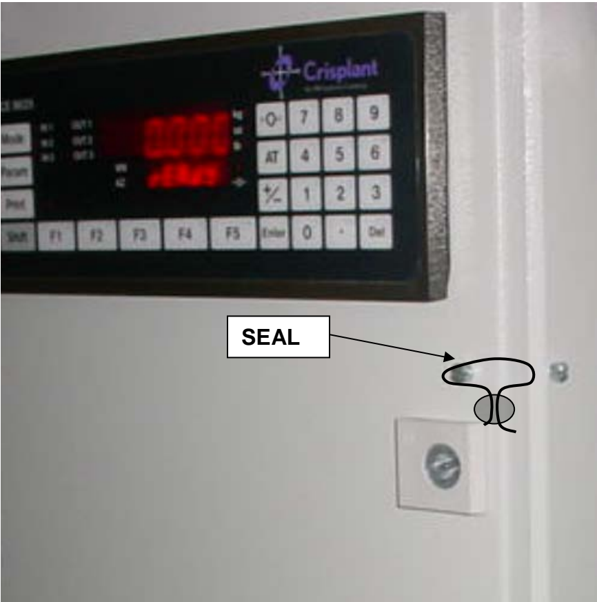
(b) Display Unit Showing Typical Sealing of The Housing
