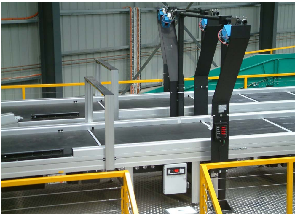
(b) FKI Logistex Model WBC-F Incorporated Into Conveyor System, With SICK Model VMS-520 (Variant 2)
